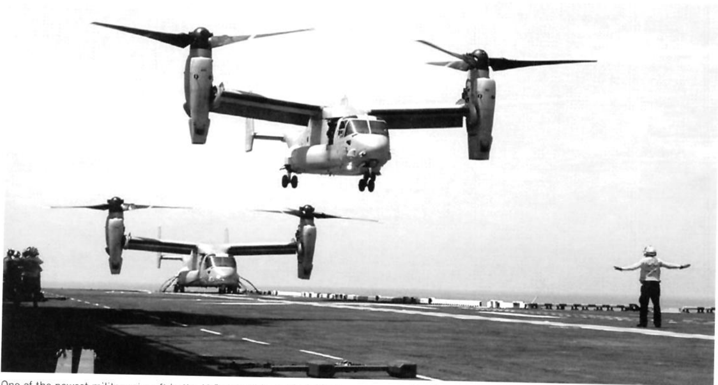
One of the newest military aircraft in the U.S. inventory is the V-22 Osprey, expected to fill the medium-lift needs of the Marine Corps for at least the next decade. With the engines positioned as shown here, the aircraft can take off and land vertically. Once airborne, the engines rotate 90 degrees forward, converting the V-22 into a high-speed turboprop aircraft. (Mike Jones)
