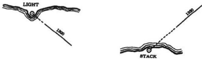
Two examples of visual gyro bearing LOPs.
