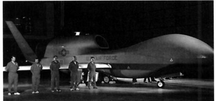
The Global Hawk UAV is a large Air Force endurance drone, able to cruise at 400 miles per hour for thirty-five hours. It can scan an area the size of the state of Illinois in just twenty-four hours. (Air Force photo)
