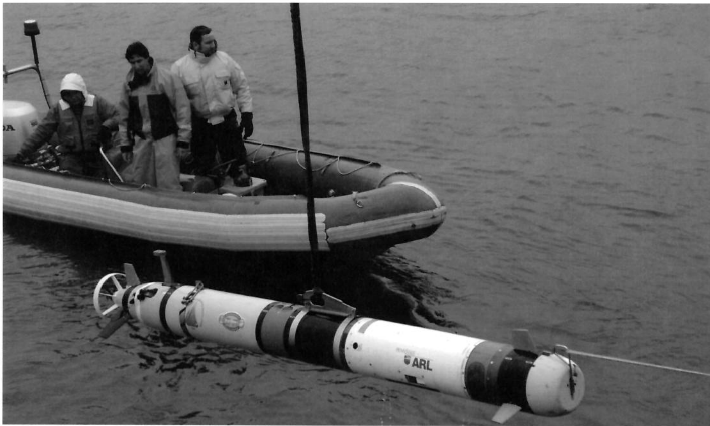
One of several models of newly developed autonomous underwater vehicles (AUVs) that can hunt for submerged mines.
