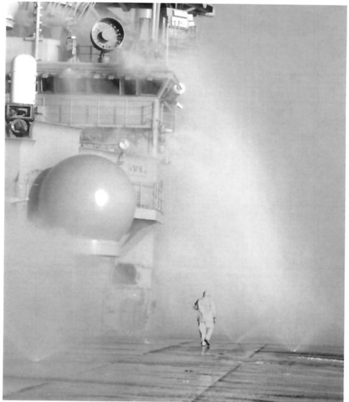
When a CBR attack is anticipated, a ship will activate the water washdown system in order to wet all exposed surfaces to make the decontamination process after the attack easier. Here, a rainbow forms as a crew member checks out the system aboard the amphibious assault ship USS Boxer (LHD 4). (Rudy Pulach)
