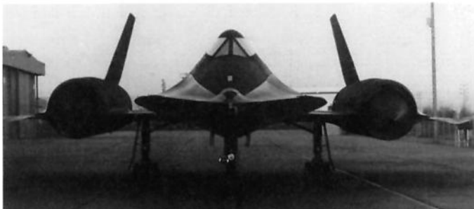
Spy planes like the SR-71 Blackbird were used extensively during the Cold War era to gather intelligence. The SR-71 could fly at altitudes above 80,000 feet at speeds in excess of Mach 3, above and beyond the effective limits of most contemporary anti-air missile systems. (Air Force photo)
