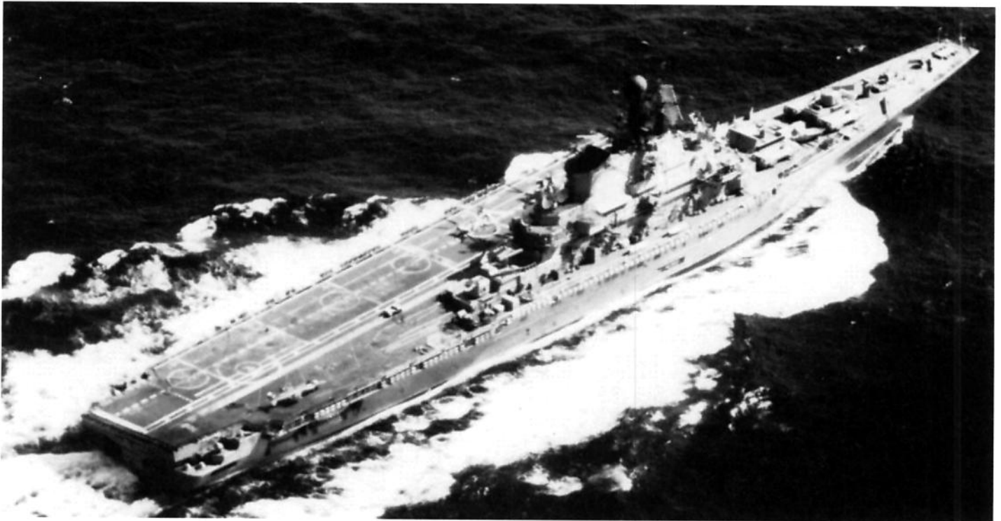
Although not the threat it once was, the Russian Kiev-class carrier Novorossiysk shown here is still a formidable warship. Note the missile launchers forward, and the VTOL fighter aircraft aft.
