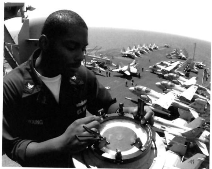
A quartermaster on the aircraft carrier USS John F. Kennedy (CV 67) uses a bearing circle to obtain a true bearing to an object. (Anthony Riddle)
