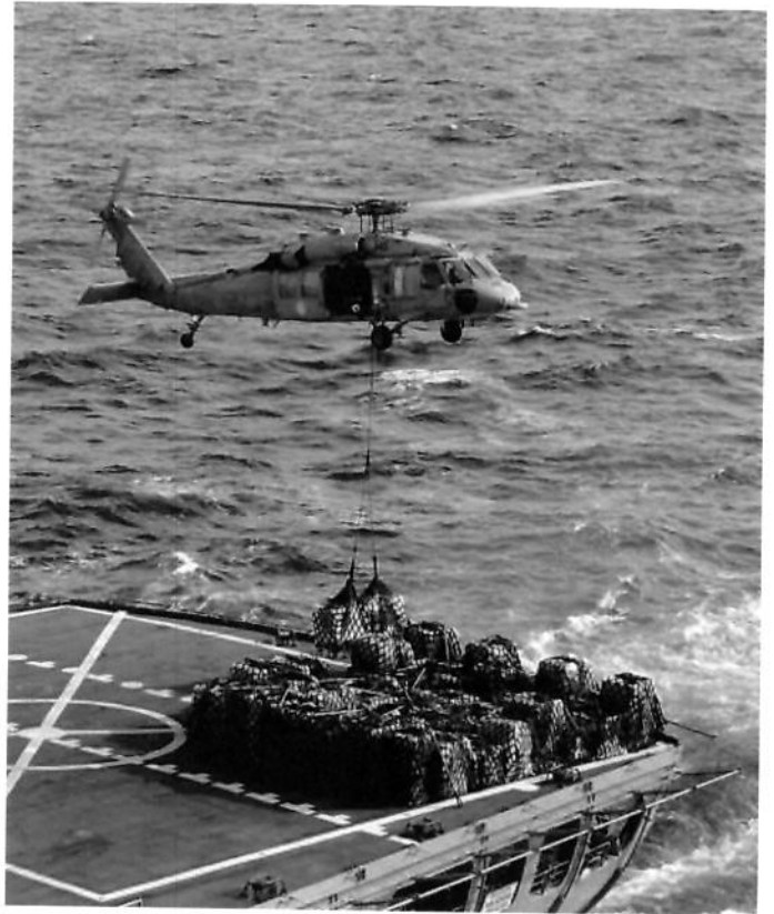
A Seahawk helicopter conducts vertical replenishment operations from an oiler. (Jessica Bidwell)
