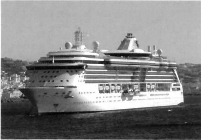
Royal Caribbean's cruise ship Brilliance of the Sea at anchor at Mykonos, Greece. With a displacement of 90,000 tons and length of 293 meters, the ship is representative of many of the newer and larger cruise ships now being placed in service. Luxury accommodations can be provided for up to 2,500 passengers. (ShipParade photo by Richard Maidment)
