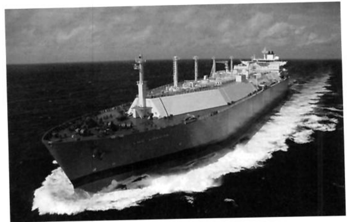
A highly sophisticated type of tanker is the liquefied natural gas (LNG) carrier, like the SS El Paso Southern shown here. They carry natural gas liquefied at -260^{\circ} Fahrenheit.
