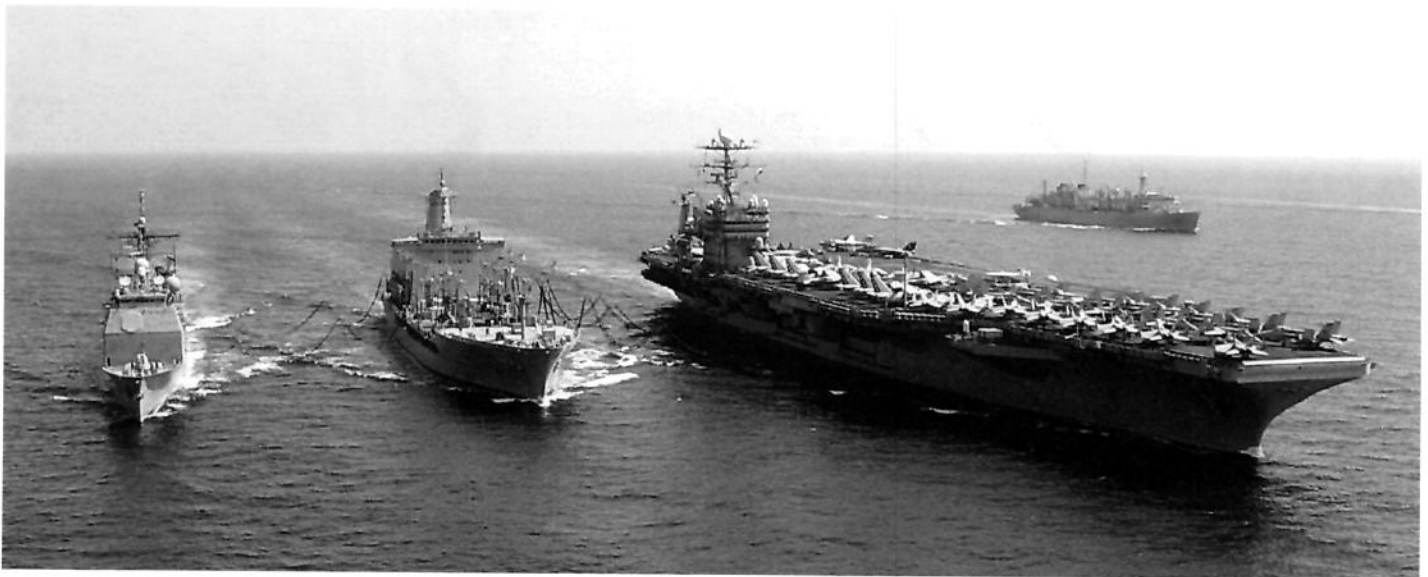
An underway replenishment operation with the oiler USNS Leroy Grumman simultaneously refueling a Navy aircraft carrier and a destroyer. The replenishment ship is USNS Supply in the background.
