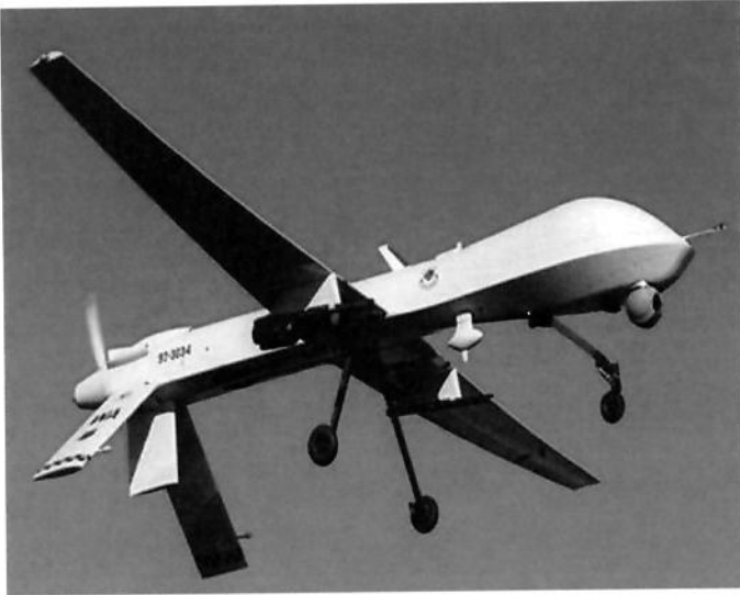
UAVs such as the Predator shown here provide real-time infrared and color video to intelligence analysts and controllers both on ships at sea and on shore, and can be fitted with smart weapons for covert attacks.
