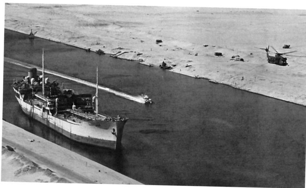
A mine countermeasure Sea Stallion helicopter tows a magnetic minesweeping sled past an Egyptian merchant ship while sweeping the Suez Canal during Operation Nimbus Star in 1974. The canal had been closed for seven years by Egyptian mines laid during the Arab-Israeli wars of the 1960s.
