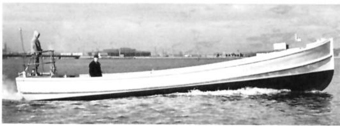
Utility boats, like this personnel boat, are used for transporting people and light equipment.
