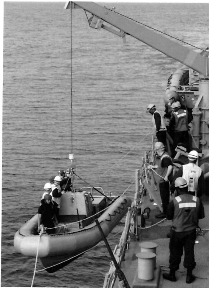
Rigid hull inflatable boats (RHIBs) have become the workhorses among the small craft of the fleet, doing duty as lifeboats, personnel boats, fast patrol craft, and utility boats.
