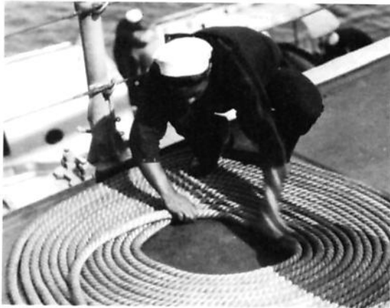
Flemishing down a line. The bitter end is in the center.
