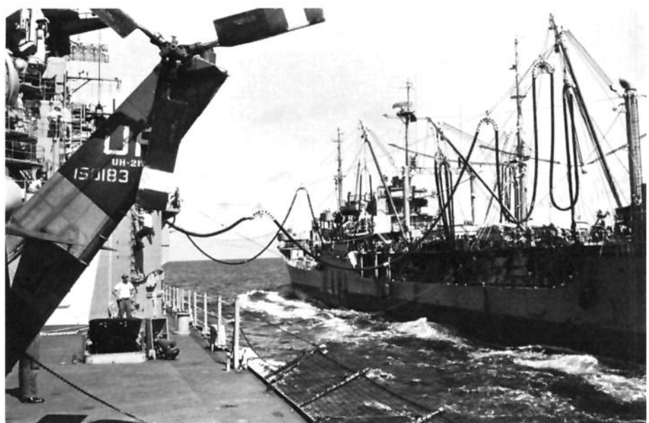
Several booms and their rigging are shown in use by this oiler during an underway replenishment of another ship alongside.
