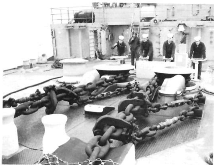
Sailors on a ship's forecastle making ready to anchor. Note the two chain stoppers securing each anchor in place.
